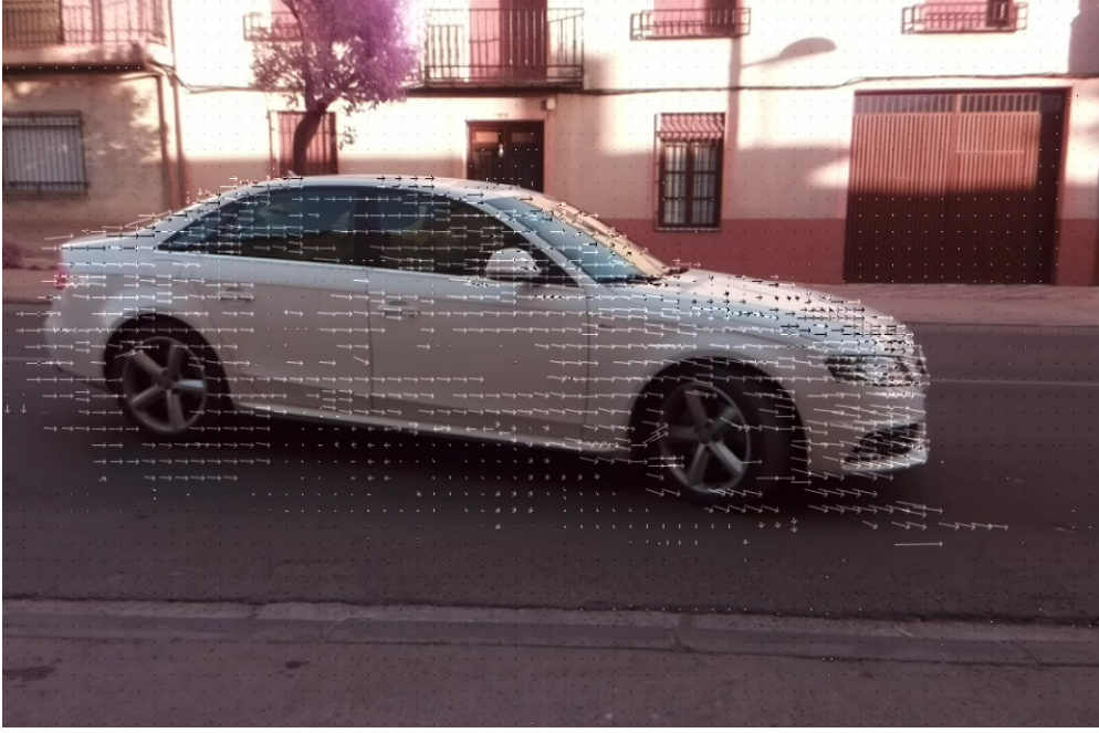
Figure 2: Example of motion vectors obtained using the developed device
